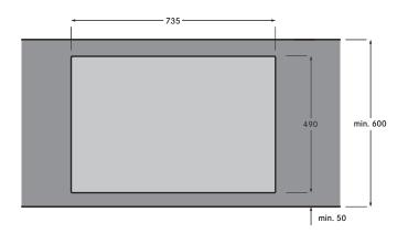
With regard to the suitability of the worktop, the instructions from the worktop manufacture must be adhered to. For example, worktop cut-outs must be appropriately sealed against moisture.
